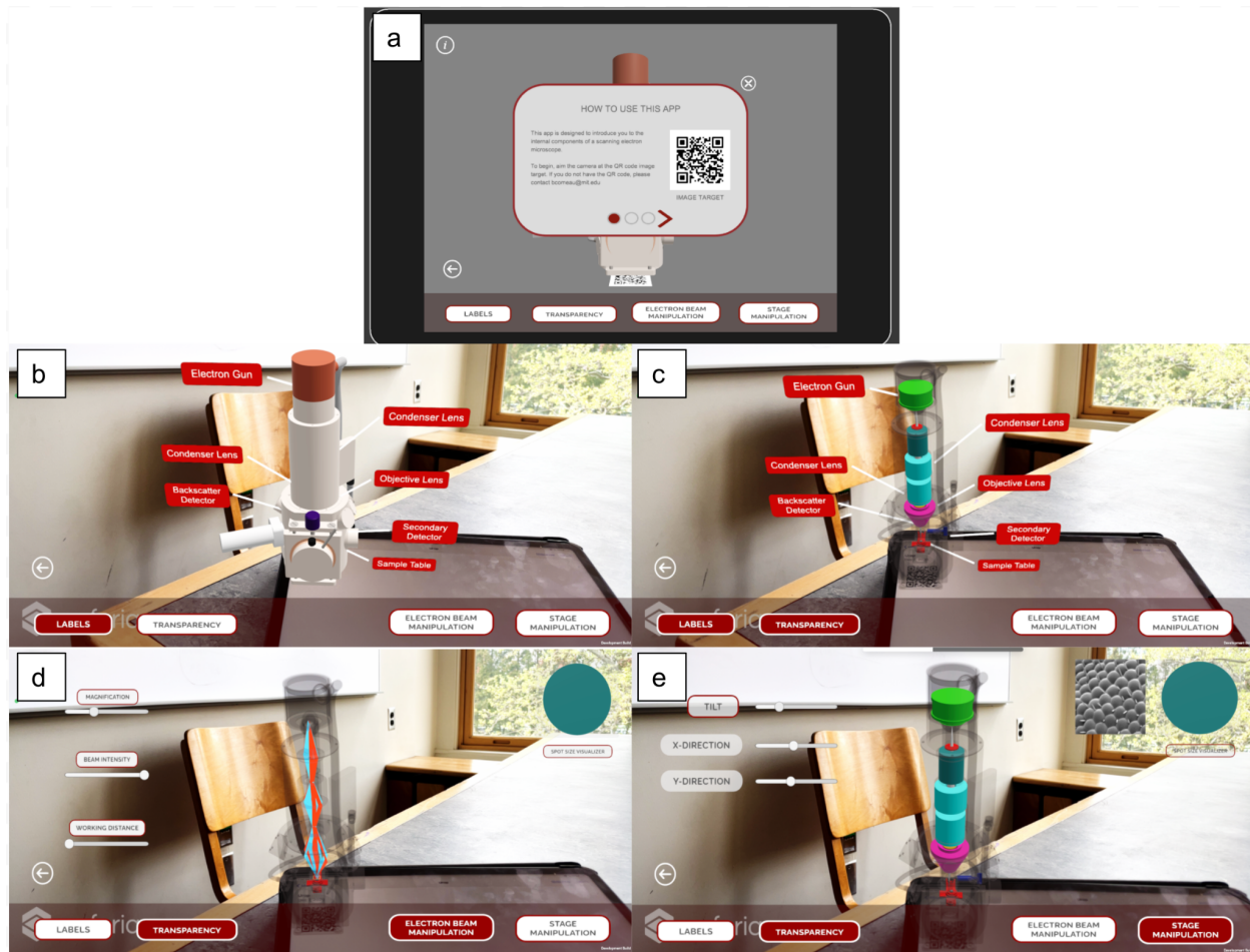
Figure 2. A flow of the UI: a) the machine introduction where users are able to toggle b) labels and c) transparency on/off throughout the activity. Additional capabilities include manipulating d) the electron beam, and e) the stage to see changes to the quality and position of the resulting image.
